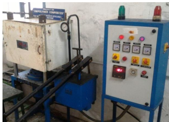
Fig 1.3 Compression moulding process
