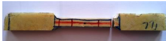
Fig1.4 preparation of tensile test specimen
