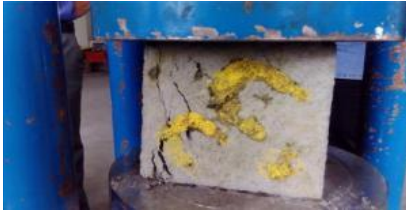
Fig.2. Cube Specimen after Failure
