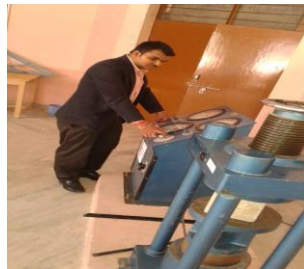
Fig.2 Testing cube for Compressing Strength by Compressive Testing Machine
