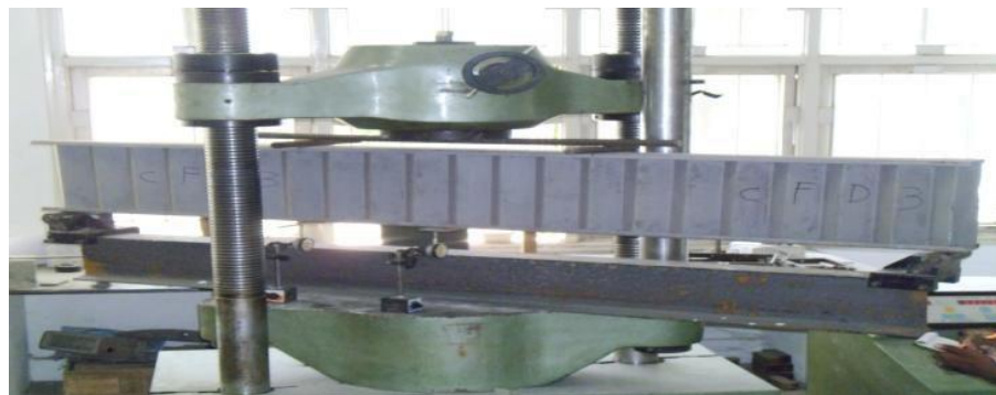
Fig. 4 Experimental testing of Cold formed steel beam.
