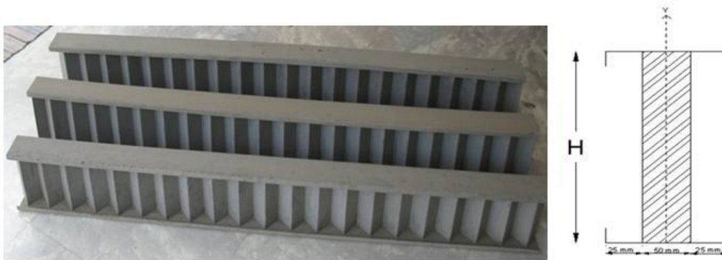
Fig. 2 Cross section and cold form steel beams with varying web depth.
