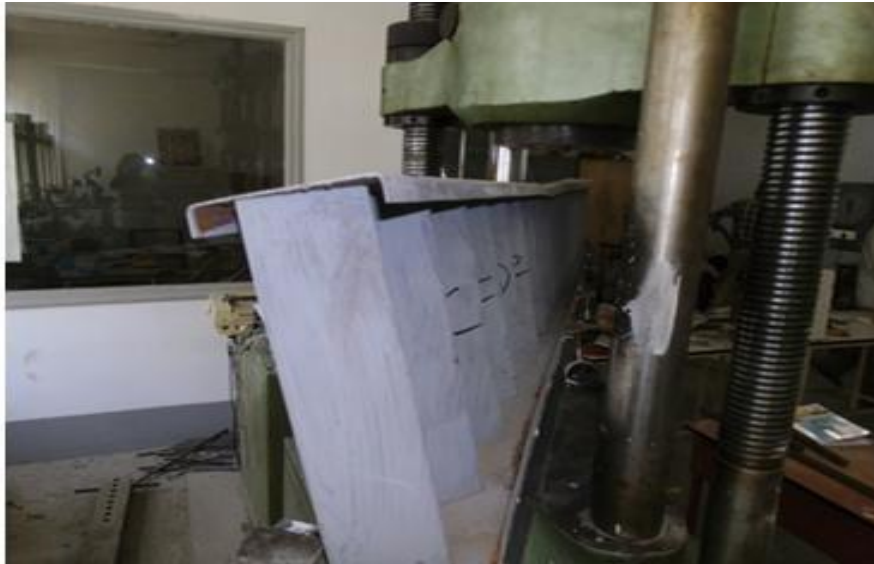
Fig. 5 Failure mode of test specimen- lateral torsional buckling.
