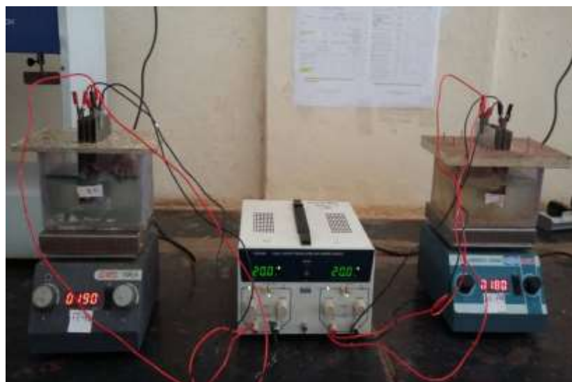
Fig2. Photo view of Experimental setup of EC process for dairy industry wastewater treatment.
