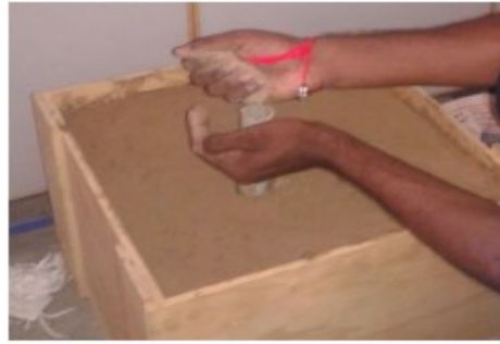
Fig 17 Filling the hole using sand
