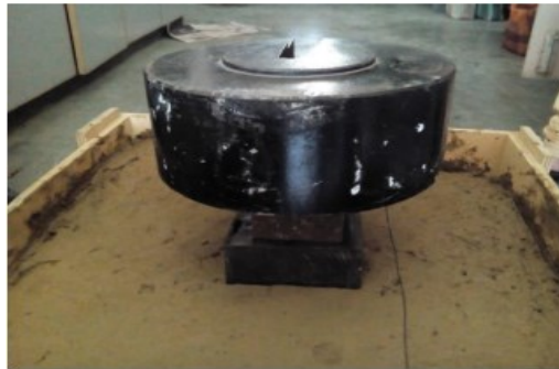
Fig 13- Application of load without the sand pile
