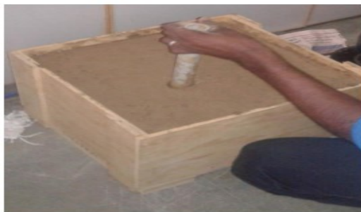
Fig 15- Drilling the hole for pile
