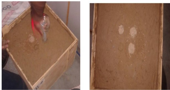
Fig 18 - Erection of sand pile in diagonal direction
