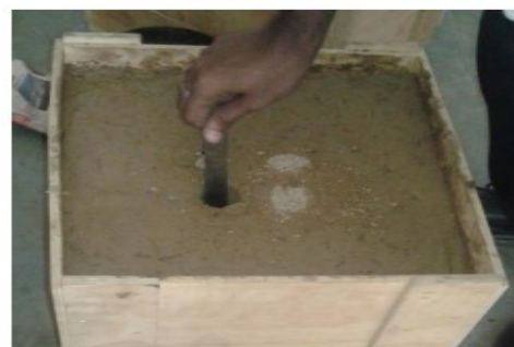
Fig 16 - Measuring the depth of pile
