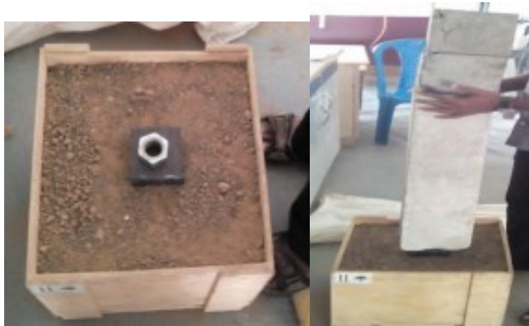
Fig 10 - Application of load over dry soil
