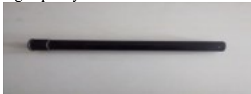
Fig 9 pipe used for drilling the soil
