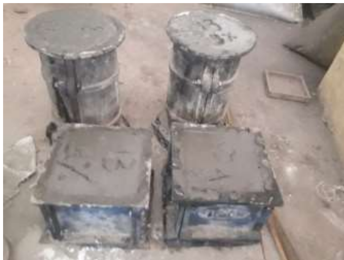
Fig 4:Casting of cubes and cylinder
