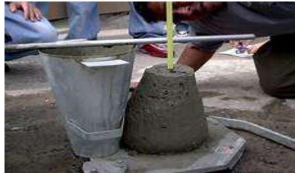
Fig 3: Slump obtained after the test
