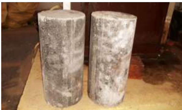
Fig 5: Cylinder Before Testing Of Split Tensile Strength
