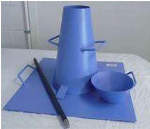
Fig 2: Slump cone test apparatus
