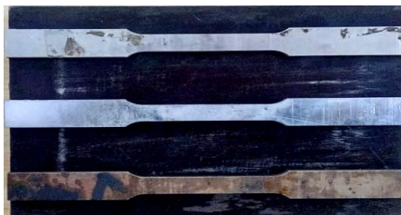
Fig 4.3 Tensile Test Specimen
