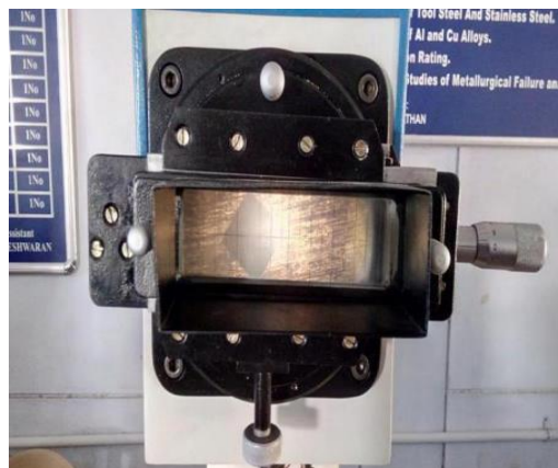
Fig4.1 Vickers hardness tester
