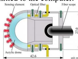
Fig. 1. Hardware structure of optical three-axis tactile sensor
