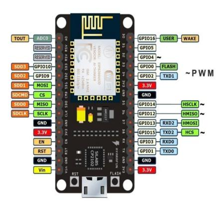
There is a candid difference between Vin and VU where former is the regulated voltage that may stand somewhere between 7 to 12 V. while later is the power voltage for USB that must be kept around 5 V.
