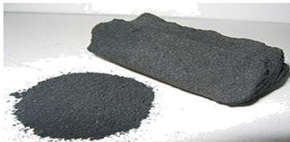
Fig no: 1 Activated carbon is used as an adsorbent
