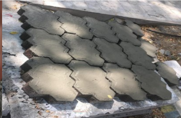
Fig 3 – casted paver blocks
