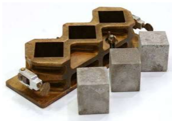
Figure: 2 Mould used for compressive test
