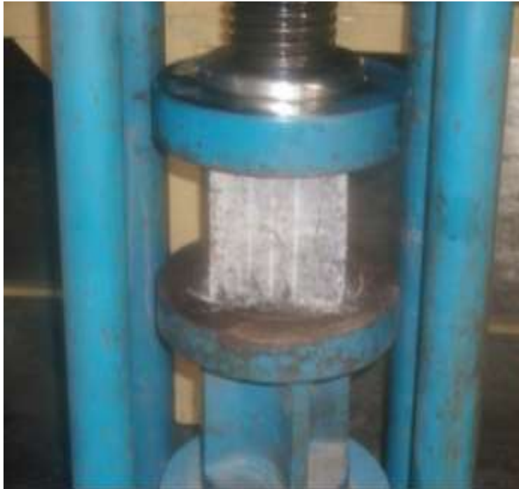
Figure: 1. Testing of Compressive strength test specimen
