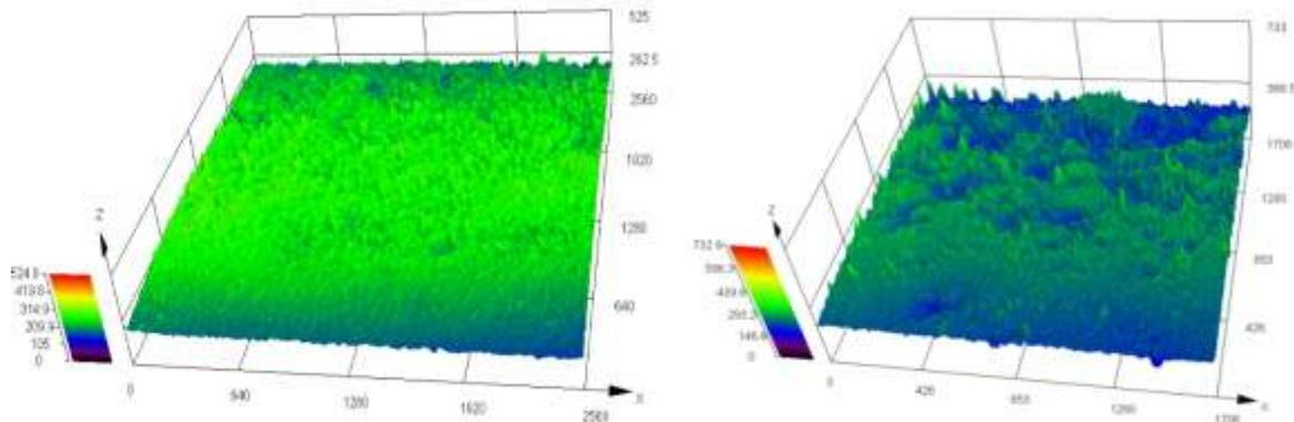
**Fig. 4** Surface texture of the cast samples, (a) Smooth surface and (b) Rough surface.
