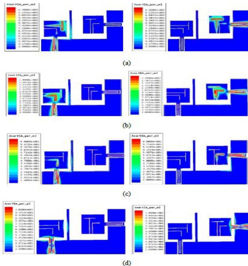
**Fig.4** (a) Current distribution at 3.32 GHz when port-1 and port-2 are excited.
