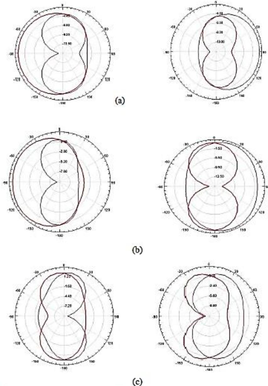
**Fig.5** (a) Radiation patterns at 4.13 GHz when port-1 and port-2 are excited.
