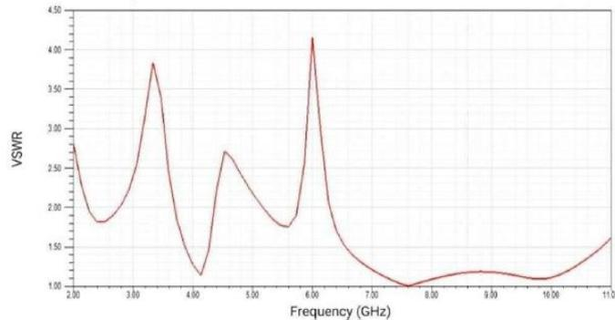
**Fig.6** Simulated VSWR characteristics
