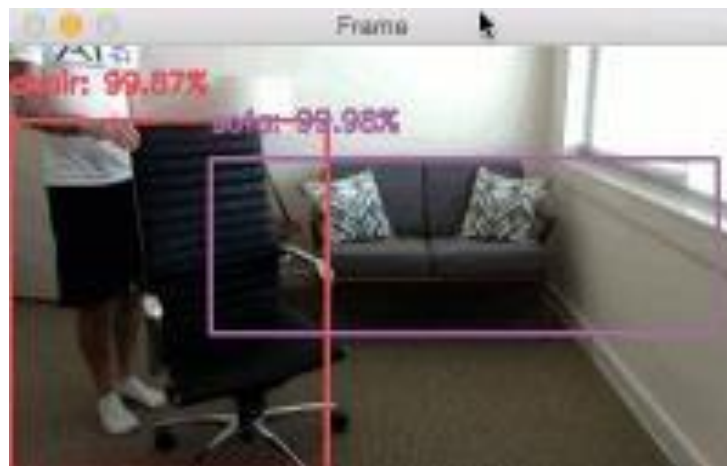
Figure 1: A short clip of real-time object detection with deep learning and OpenCV + Python
