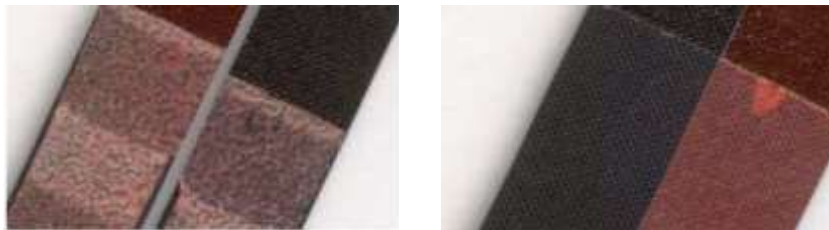
Fig. 8. Cohesive (left) and adhesive (right) failure of bonded joint [16].
