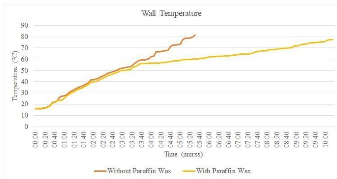
Figure 8: Temperature-time distribution with different \Psi of PCM at 3.68 kW/m 2 for finned array heat sink
