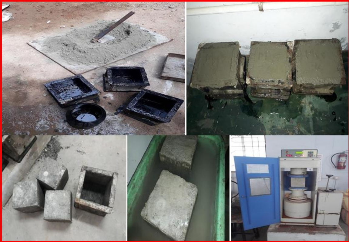
Fig.5. Mixing, Casting & Testing of Cube Specimens
