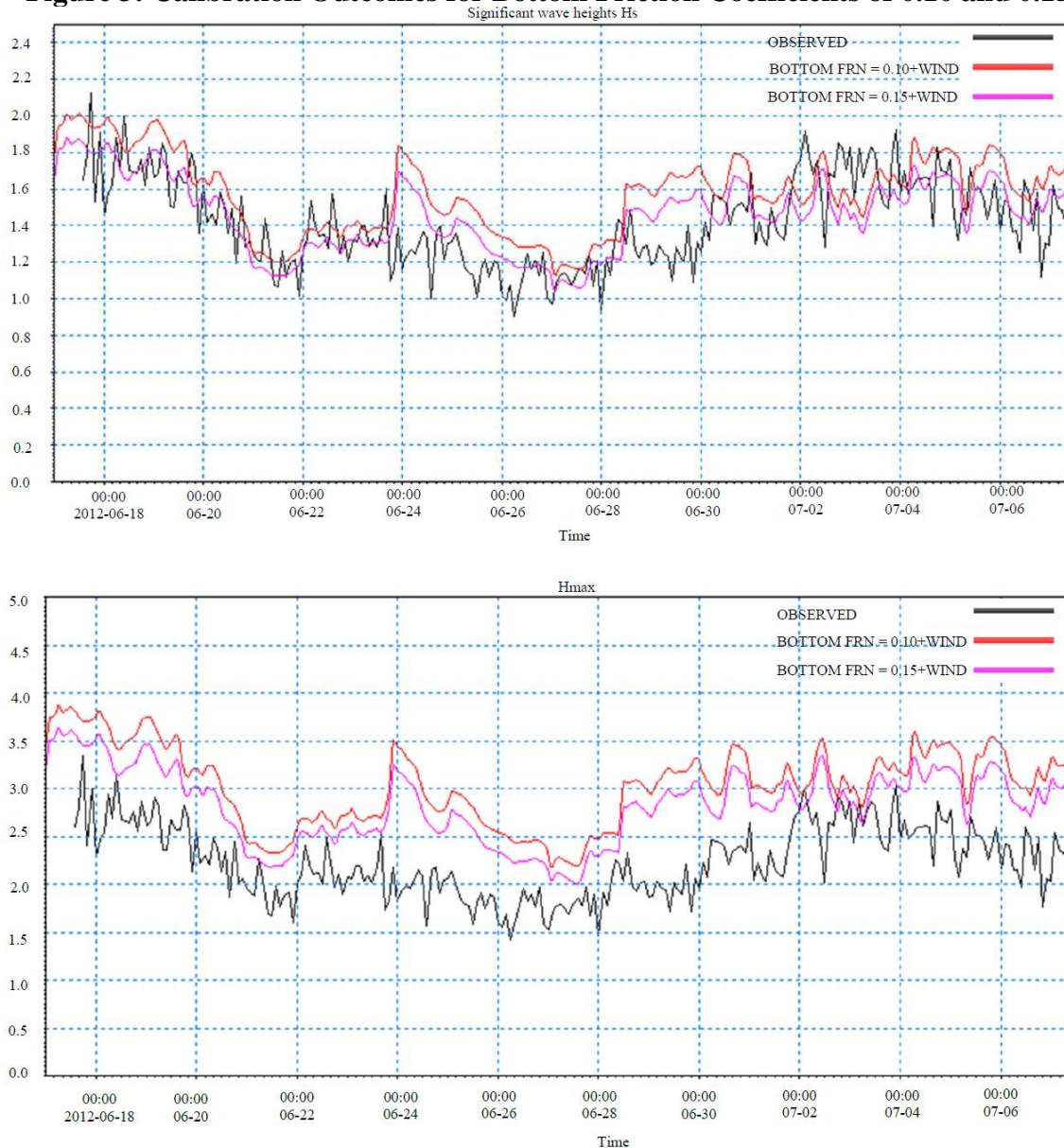
Figure 3: Calibration Outcomes for Bottom Friction Coefficients of 0.10 and 0.15
