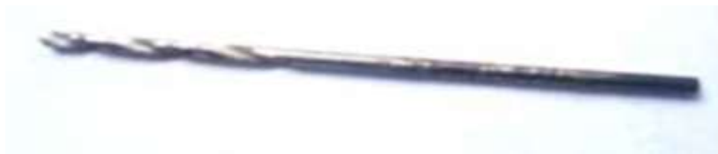
Fig. 4. TiCrN coated micro drill bit
