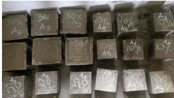
Fig.1. Concrete cubes made with different mix proportions
